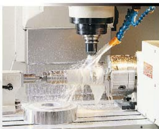
High pressure coolant (P:3.5 kg/cm 2 , Q:100 l/min)
