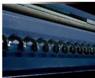
Automatic chip removal (Screw type chip conveyor)
